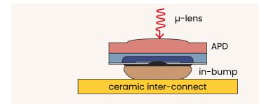
HgCdTe APD technology flip-chip hybridized onto a ceramic interconnection circuit and back-side illuminated through a monolithically integrated microlens.
