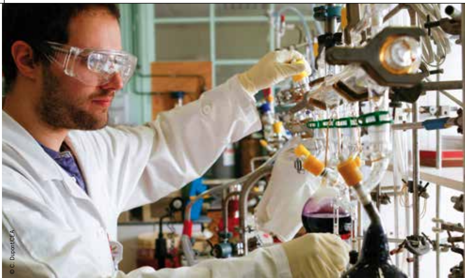
Chemical manipulations on a vacuum gas manifold.
